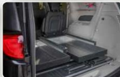
Stow 'N Go® seating and two aluminum floral trays are accessible when the hinged casket floor is folded over.
