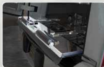
Two 90-degree rollers, a chrome-plated Extend-A-Sill, and a quick-release bier pin complement the exquisite interior.
